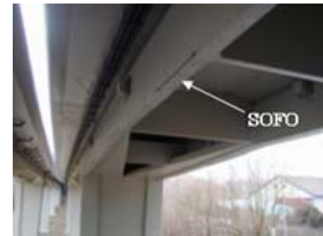
Deformation measurement of a concrete bridge deck
