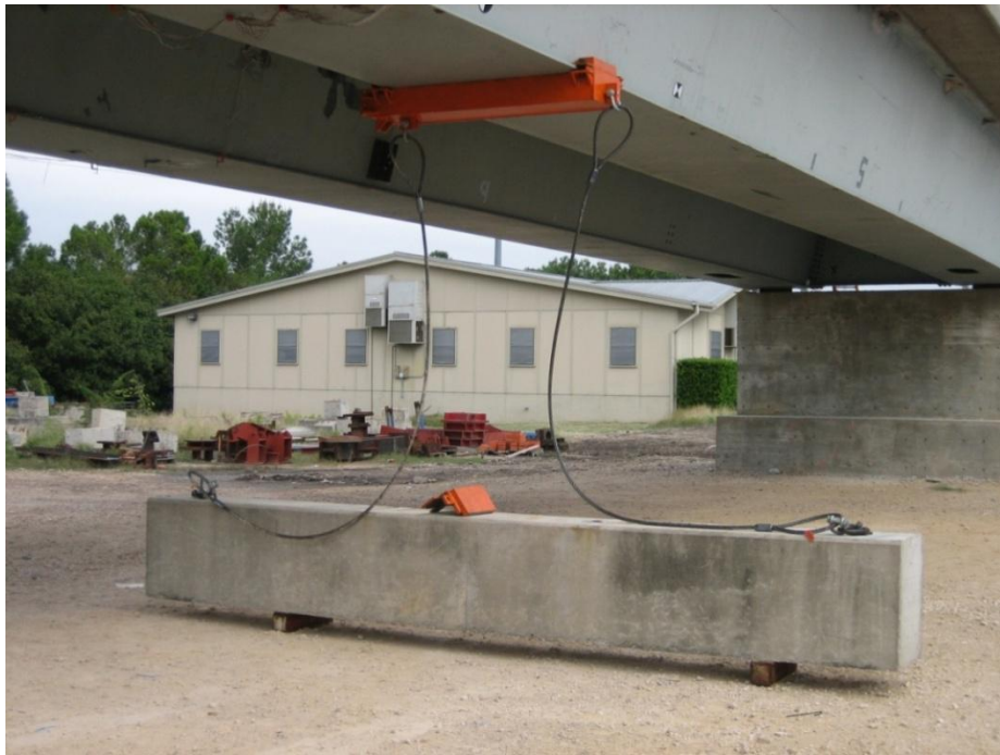
Figure 3. Explosive shaped charge applied to test bridge
