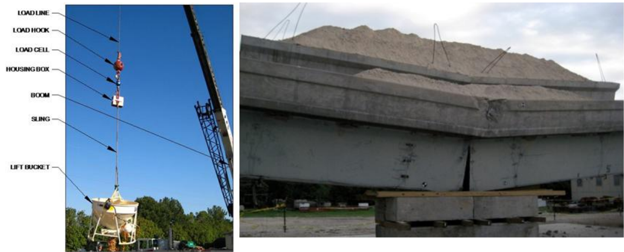
Figure 12. Bridge loaded to collapse.
